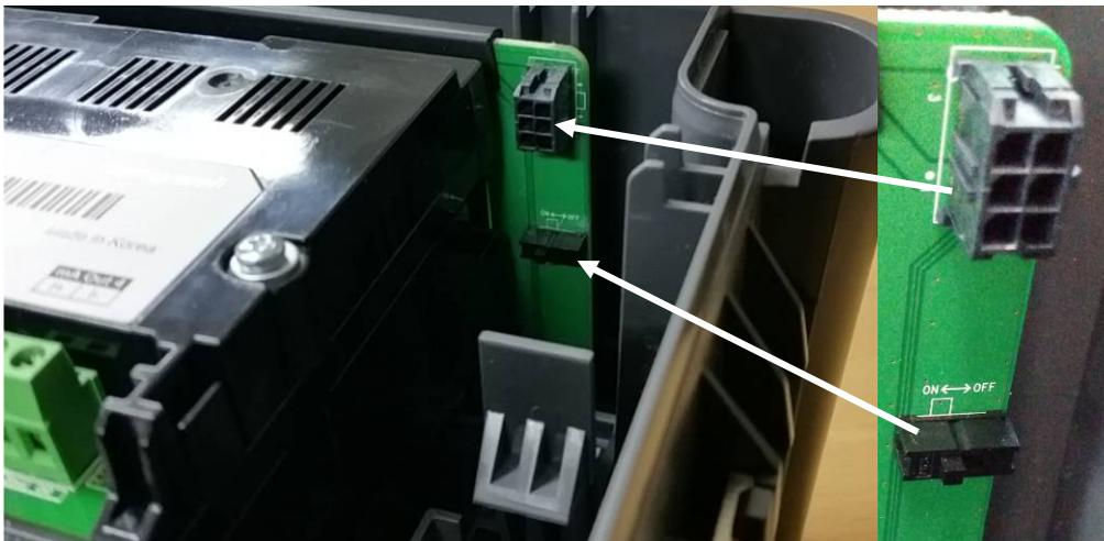
Figure 18. Battery On/Off Switch and Battery Connector
